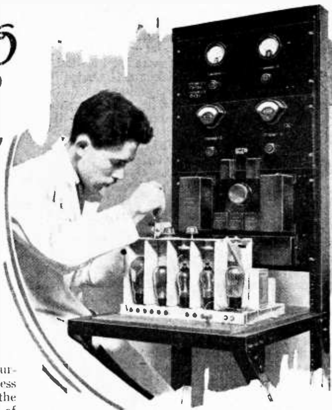
Front view of the apparatus for testing the audio-frequency response of a completed receiver.
