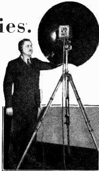
SETTING A SPEECH TRAP. An American "O.B." engineer with the parabolic microphone recently tested in the Washington Senate House with a view to the inauguration of political broadcasts.
